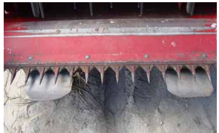
Figure 3. Relay plant depressants in front of cutting bar to avoid cutting etiolated seedlings of relay crops between 14" spaced barley rows.
